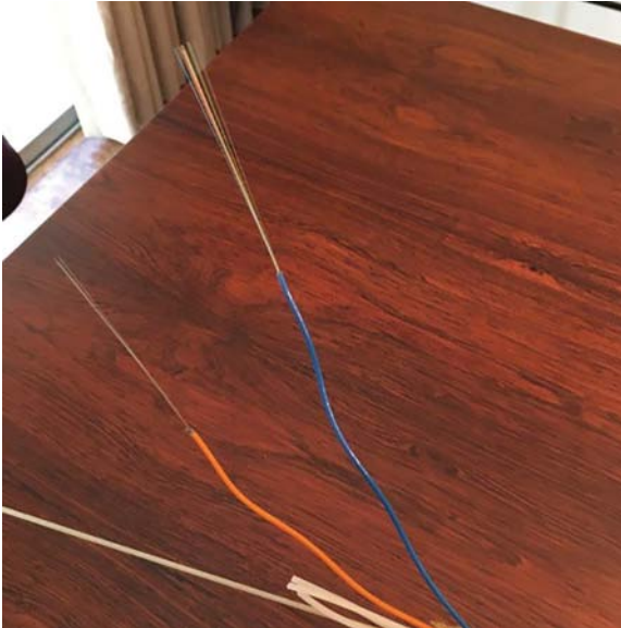
Figure 1-3 Examples of fiber-optic cabling used in telephone company networks. (Photo by Annabel Z. Dodd)
